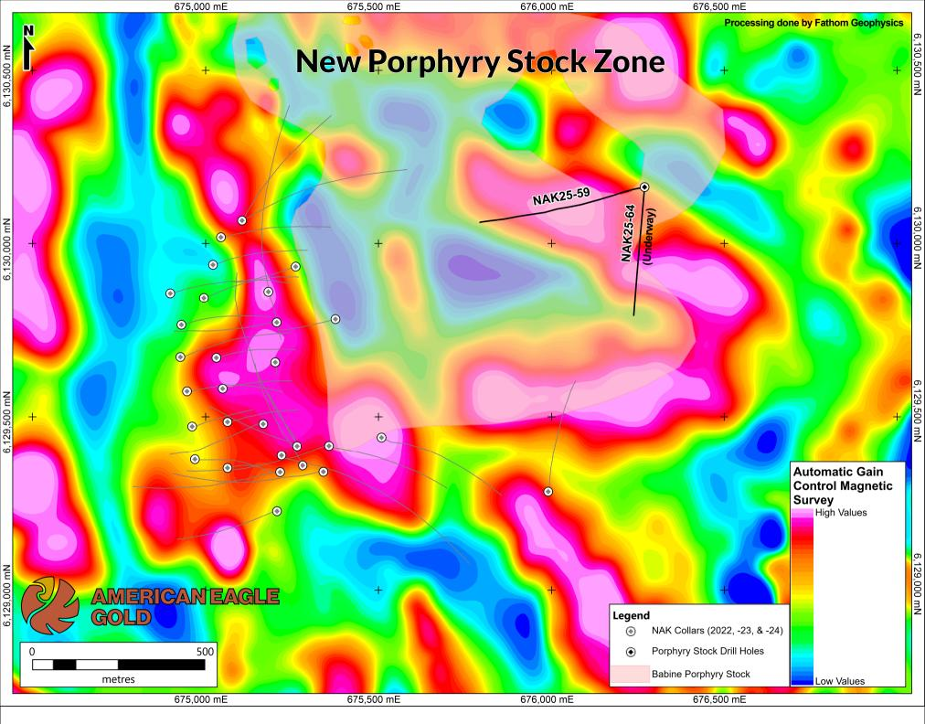
The automatic gain control filter (AGC) is a means of evening out the amplitudes of anomalies. This makes more subtle features in the data visible. The filter also acts as a high-pass filter by suppressing the longer wavelengths.
