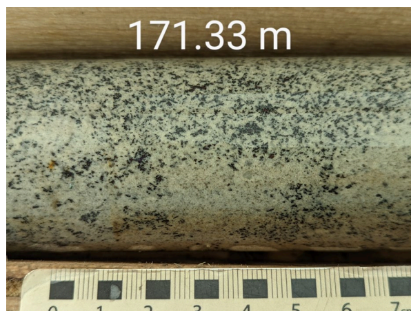
NAK23-12: Bleached monzonitic dyke with densely disseminated bornite
