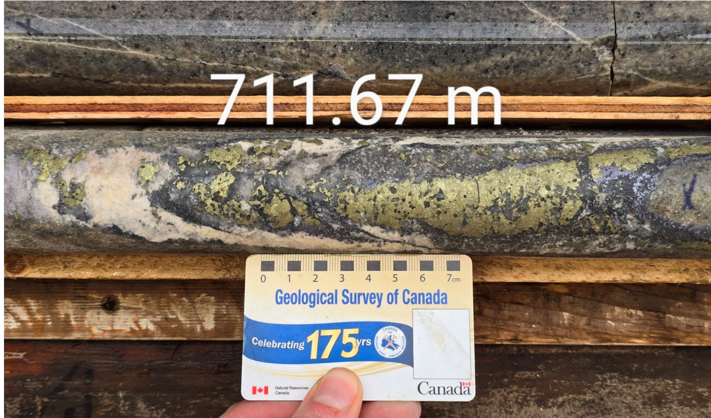
Quartz vein with chalcopyrite and molybdenite from 711.67m in NAK24-30.
